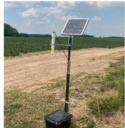
Fig. 1. Rotating arm impaction sampler deployed in a commercial potato field in 2023.
